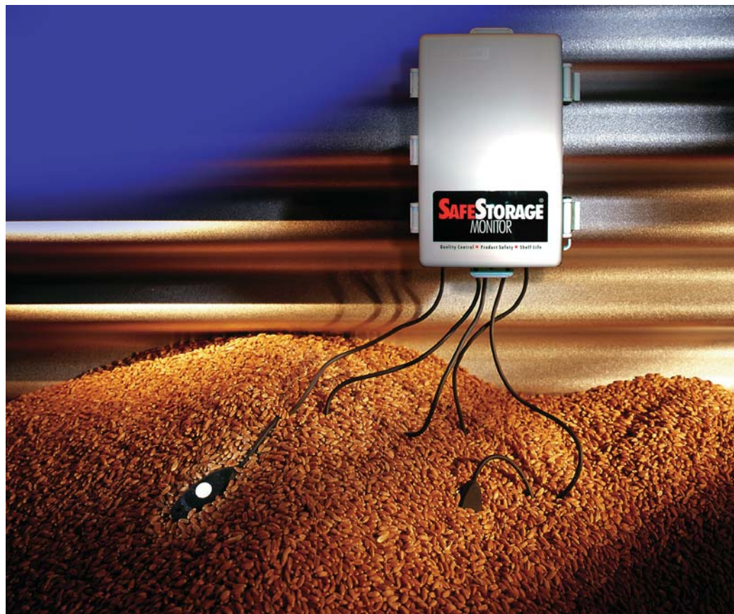
■ 5-channel data logger for long-term, unattended water activity monitoring.
